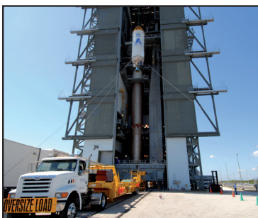
Upper stage being mounted onto the Atlas V booster, Cape Canaveral (Image Courtesy NASA)
