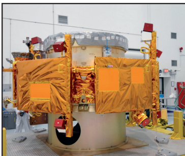
LCROSS payload being prepared for launch (Image Courtesy NASA)
