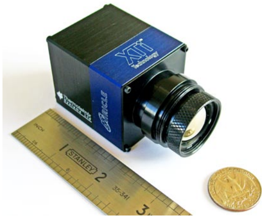
FIGURE 3. Elimination of thermo-electric heater-cooler hardware and shutterless operation allows the Thermoteknix MIRICLE 110KS thermal imaging camera to fit into a minimal volume, compact, ruggedized package. (Courtesy of Thermoteknix)
